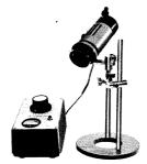
nator Base X-DE, the Illuminator supplies transmitted light. Focusing is adjustable by shifting the bulb filament. A 6V to 8V variable transformer is provided. Eight filters are available in various sizes, including color, black and white neutral density etc. for transparent or translucent subjects.
